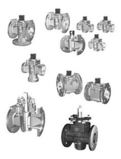
The oldest design of valve comprising of a body with a tapered, or less frequently, a parallel plug. Design variants include Non-lubricated, Fluoropolymer sleeved, Lubricated and Pressure balanced designs. Principally designed for on/off isolation of fluids they have inherent quick opening flow characteristics similar to ball valves, although specially designed eccentric plug designs may be used for flow control applications.
