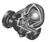
**Ball Float Steam Trap (Flanged) FT-14**The FT 14 is an SG iron ball float steam trap with integral automatic air venting facility and flanged connections. It is available with horizontal connections with flow from right to left FT 14 (R-L), from left to right FT 14 (L-R). Vertical connections with flow downwards FT 14(V) is a site modified
